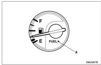
The gauge shows the amount of fuel in the fuel tank when the ignition key is turned to the "on" position. The arrow A indicates that the fuel lid (fuel filler port) is located on the right side of the vehicle. (Refer to "Fuel filler" on page 39.)
